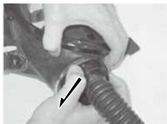
Removing of Exhalation Valve cover (In case of Model SV)
